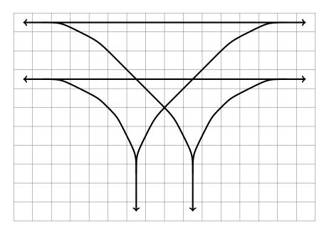
The lazy method would be to set up the entire junction as a single track section - you only need 6 TCBs for that. However, a train passing through would occupy the entire junction, even when two trains could use the junction at the same time - for example, a train going from east to west and another one from west to east. This can be solved by a slightly more complicated setup with four sections, each shown below with a different color:
