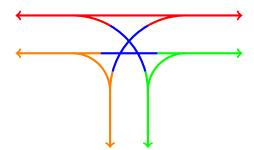
It is also possible to build the junction on multiple levels. This is known as grade separation. Note that grade-separated junctions may appear less realistic because slopes are significantly steeper than their real-life counterparts.
